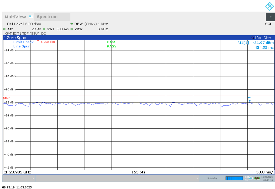
Figure 29 Spurious Emissions (Lower Band Edge 2690-2691MHz) – 64QAM (2546.01/2645.01MHz) (100MHz+90MHz Channel BW)
