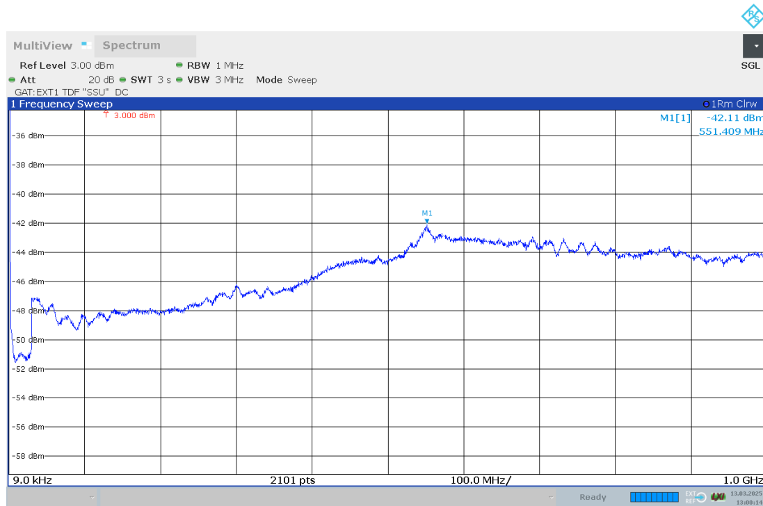
Figure 24 Spurious Emissions (9kHz–1GHz) – 16QAM (2588.01/2598MHz) (2x10MHz Channel BW)
