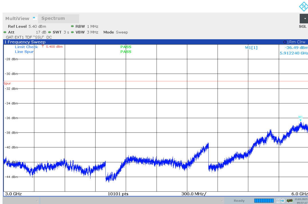
Figure 38 Spurious Emissions (3GHz-6GHz) – QPSK (2516.01/2543.49/2682.51MHz) (40+15MHz LE+15MHz UE Channel BW)
