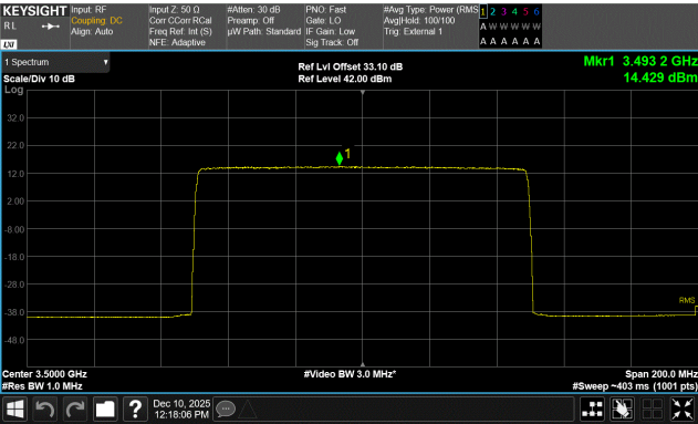
Port 1 100 MHz Channel Bandwidth 64QAM Modulation Middle Channel, 3500.01 MHz
