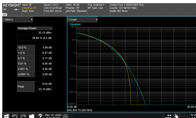
Port 1 70 MHz Channel Bandwidth QPSK Modulation Low Channel, 3485.01 MHz
