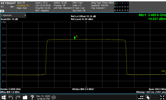
Port 1 100 MHz Channel Bandwidth QPSK Modulation Middle Channel, 3500.01 MHz
