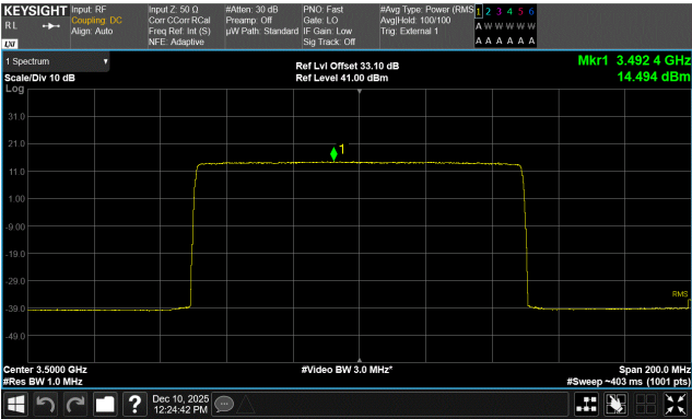
Port 1 100 MHz Channel Bandwidth 256QAM Modulation Middle Channel, 3500.01 MHz
