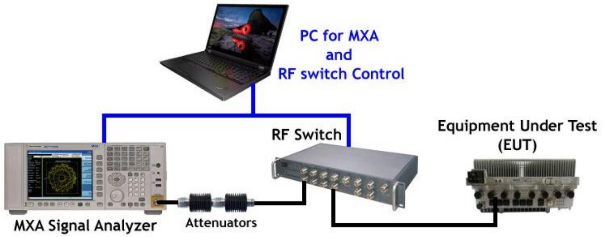
Test Setup for all Antenna Port Measurements
