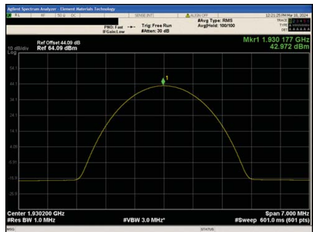
2G GSM/EDGE Band 2 8PSK Modulation Low Channel, 1930.2 MHz
