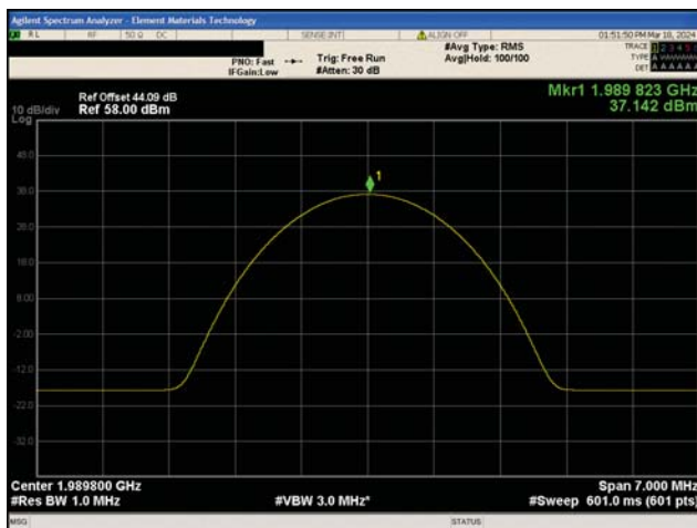
2G GSM/EDGE Band 2 GMSK Modulation High Channel, 1989.8 MHz - Reduced Power
