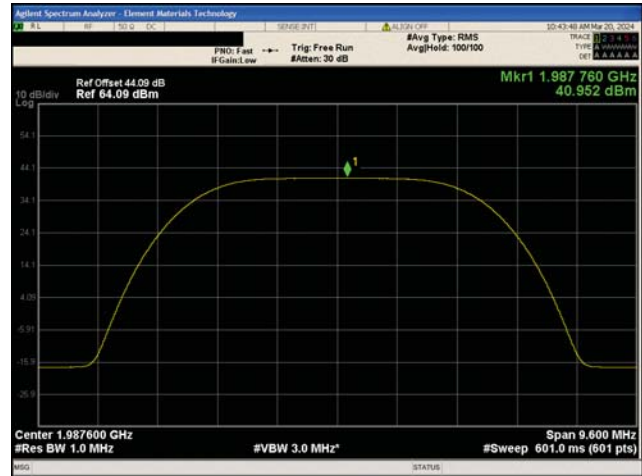
3G WCDMA PCS Band II 16QAM Modulation High Channel, 1987.6 MHz
