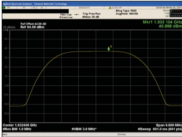
3G WCDMA PCS Band II QPSK Modulation Low Channel, 1932.4 MHz
