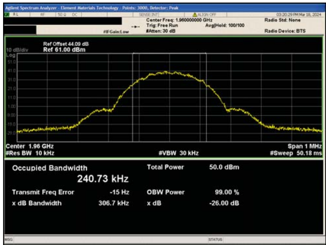
2G GSM/EDGE Band 2 8PSK Modulation Mid Channel, 1960.0 MHz
