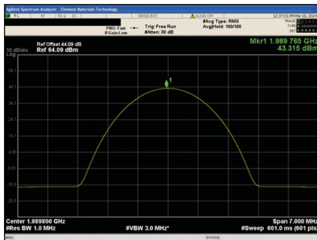
2G GSM/EDGE Band 2 8PSK Modulation High Channel, 1989.8 MHz
