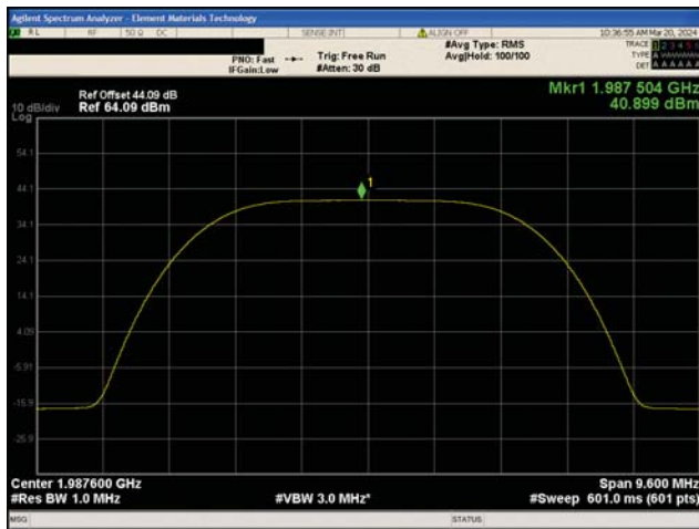
3G WCDMA PCS Band II QPSK Modulation High Channel, 1987.6 MHz
