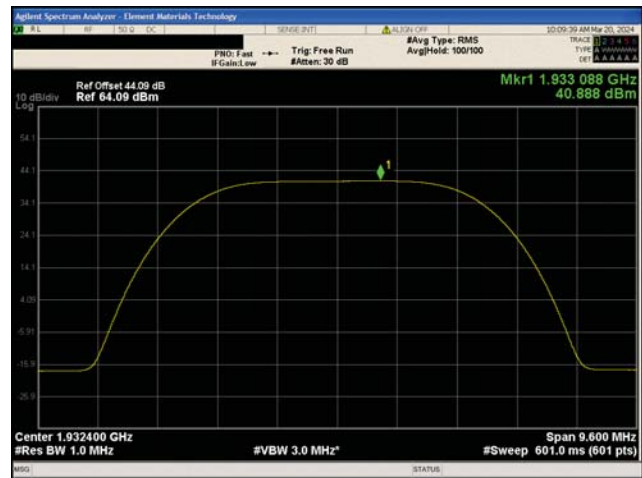
3G WCDMA PCS Band II 16QAM Modulation Low Channel, 1932.4 MHz
