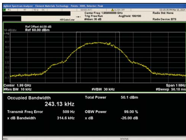
2G GSM/EDGE Band 2 GMSK Modulation High Channel, 1989.8 MHz
