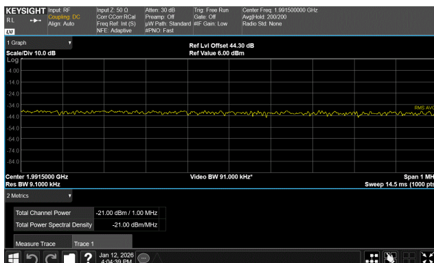
2G GSM/EDGE Multicarrier Test Case 3 8PSK Modulation 1991 MHz - 1992 MHz
