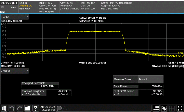
5G NR Band n85 5 MHz Channel Bandwidth QPSK Modulation High Channel, 743.5 MHz
