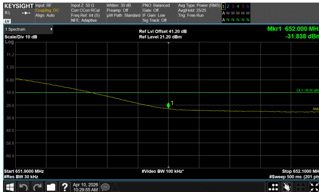
QPSK Modulation, 5 MHz channel Bandwidth 5G-NR Band n71 High Channel, 649.5 MHz 651.9 MHz to 652.1 MHz
