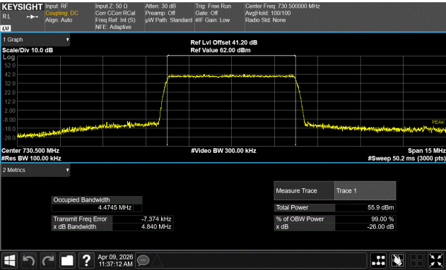
5G NR Band n85 5 MHz Channel Bandwidth QPSK Modulation Low Channel, 730.5 MHz
