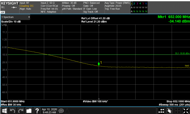
QPSK Modulation, 5 MHz channel Bandwidth LTE Band 71 High Channel, 649.5 MHz 651.9 MHz to 652.1 MHz
