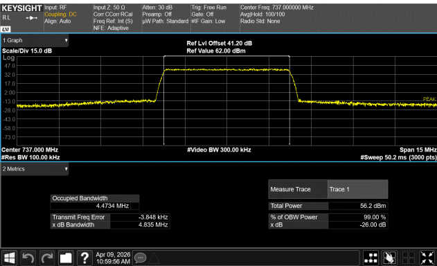
5G NR Band n85 5 MHz Channel Bandwidth 64QAM Modulation Middle Channel, 737.0 MHz
