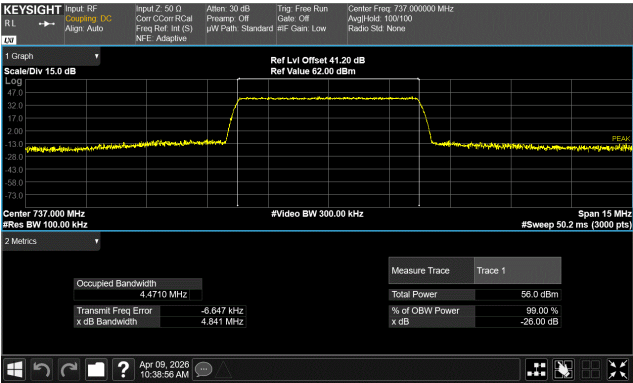
5G NR Band n85 5 MHz Channel Bandwidth QPSK Modulation Middle Channel, 737.0 MHz
