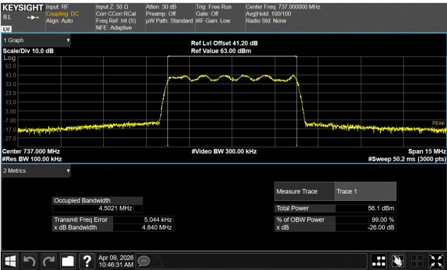
5G NR Band n85 5 MHz Channel Bandwidth 16QAM Modulation Middle Channel, 737.0 MHz
