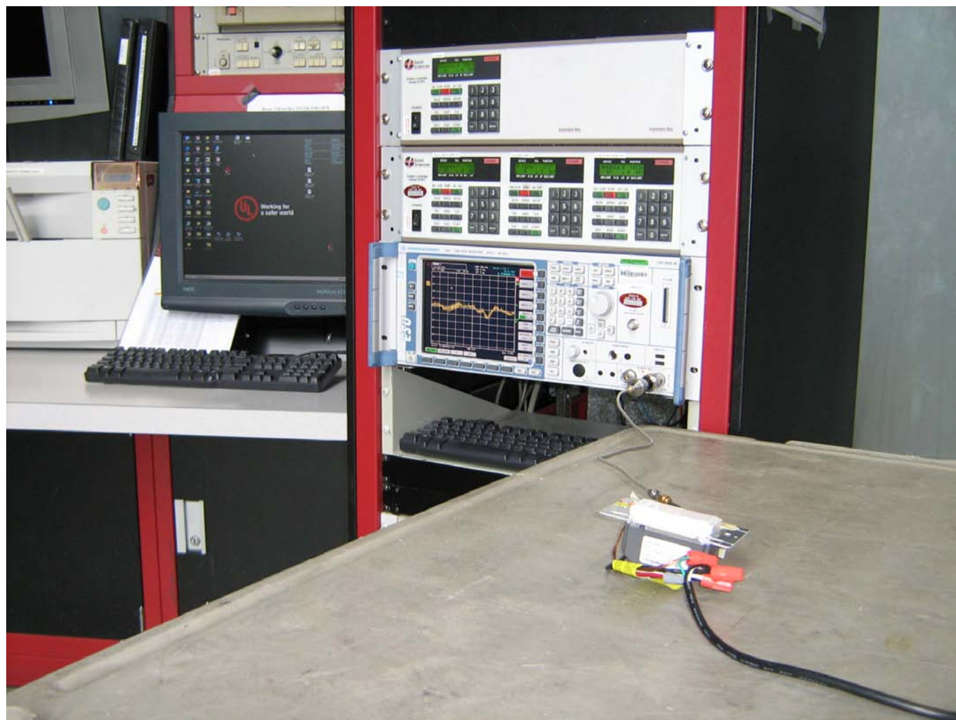
Figure 24 Test setup for Maximum Peak Output Power
