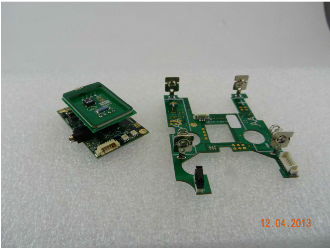
Antenna board mounted on main board with secure board
