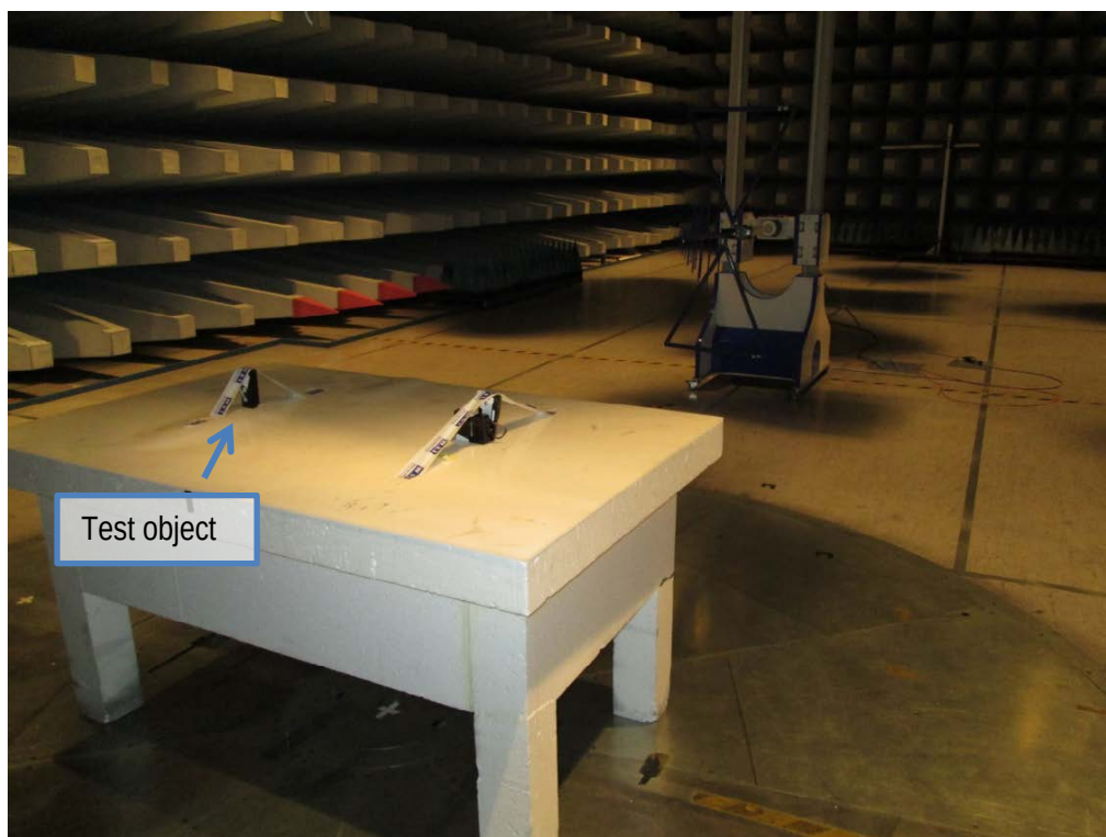
Photo 4.2.2 Test setup regarding measurement of radiated emission 30 – 1000 MHz
