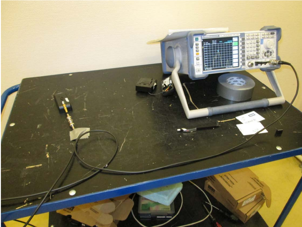
Photo 4.6.1 Test setup regarding measurement of carrier frequency stability.
