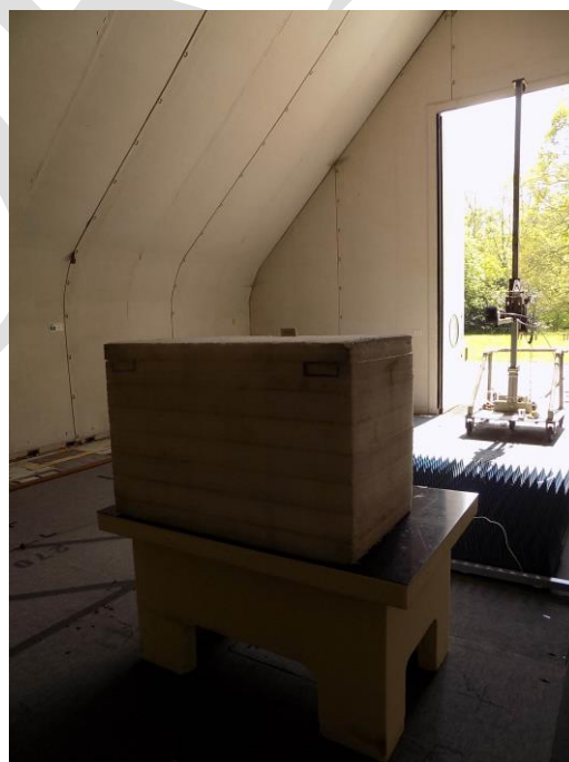
Radiated emissions, OATS, > 1000 MHz; 29L
