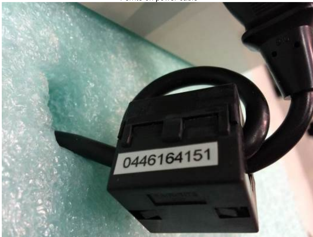
Ferrite on power cable
