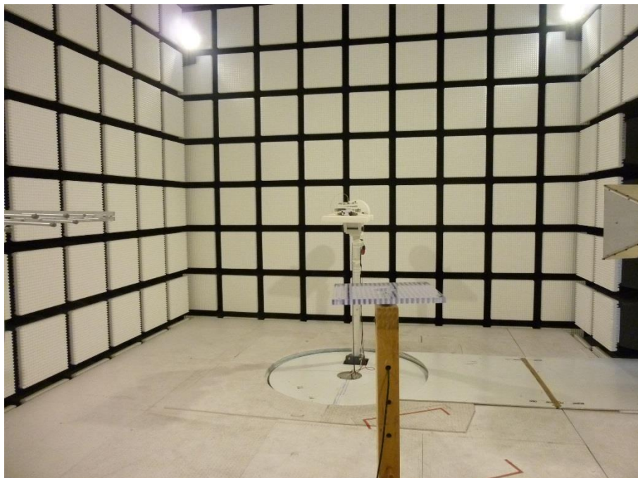
Photo 18: EUT at the anechoic chamber with spoiler antenna
