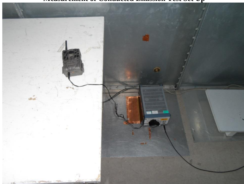
Measurement of Conducted Emission Test Set Up
