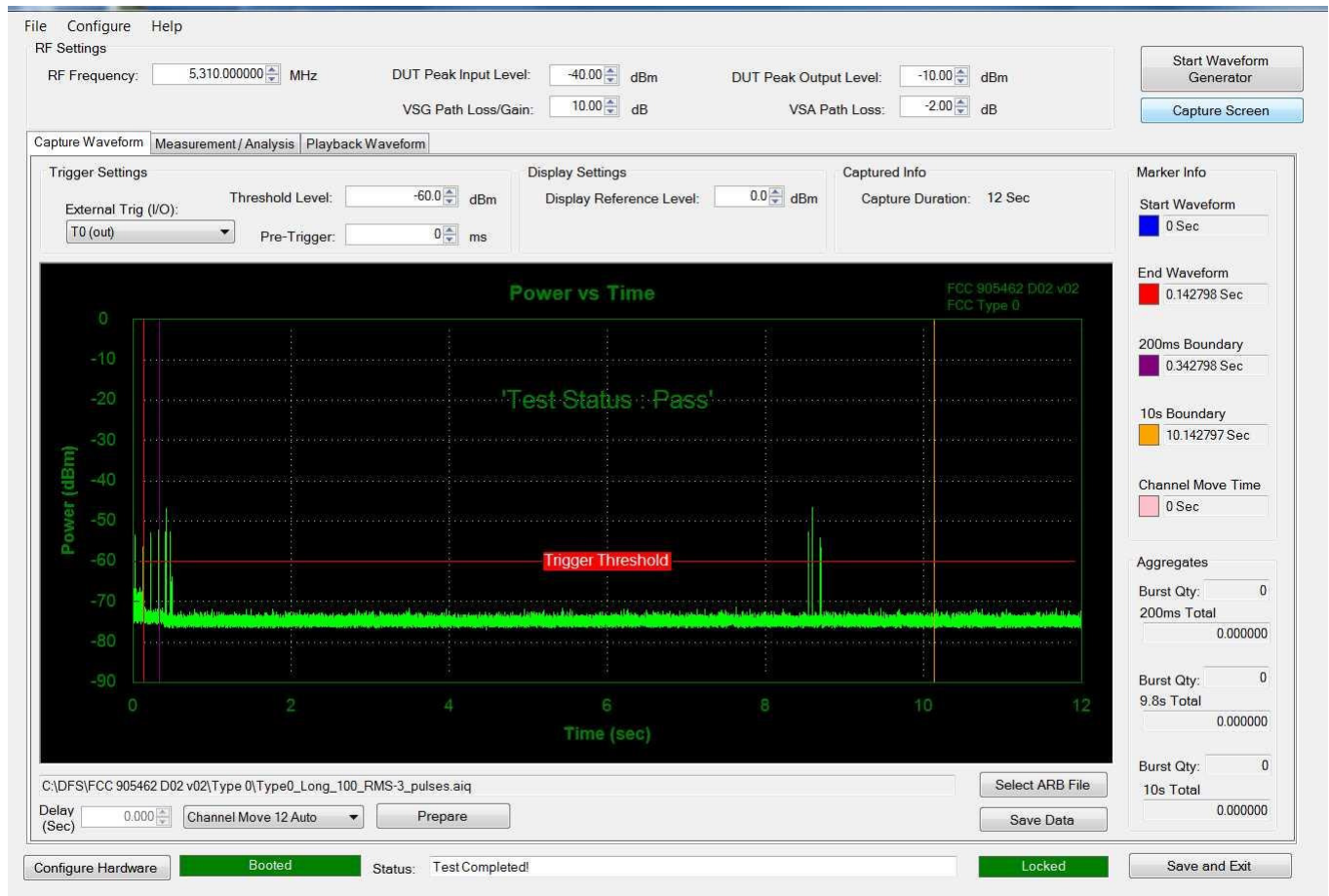
Figure 8.6-1: Channel closing transmission and move time, U-NII-2A band
