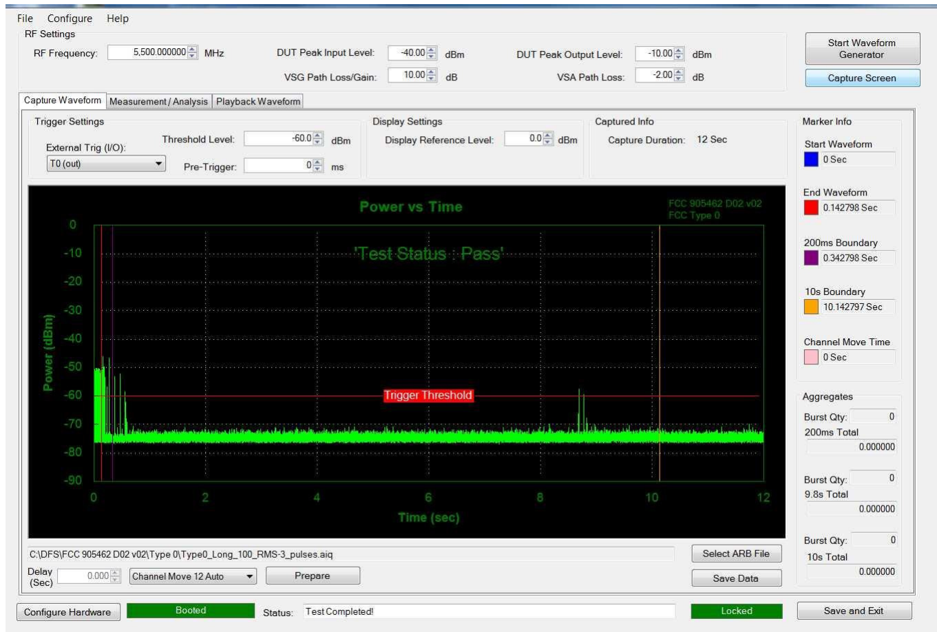
Figure 8.6-2: Channel closing transmission and move time, U-NII-2C band
