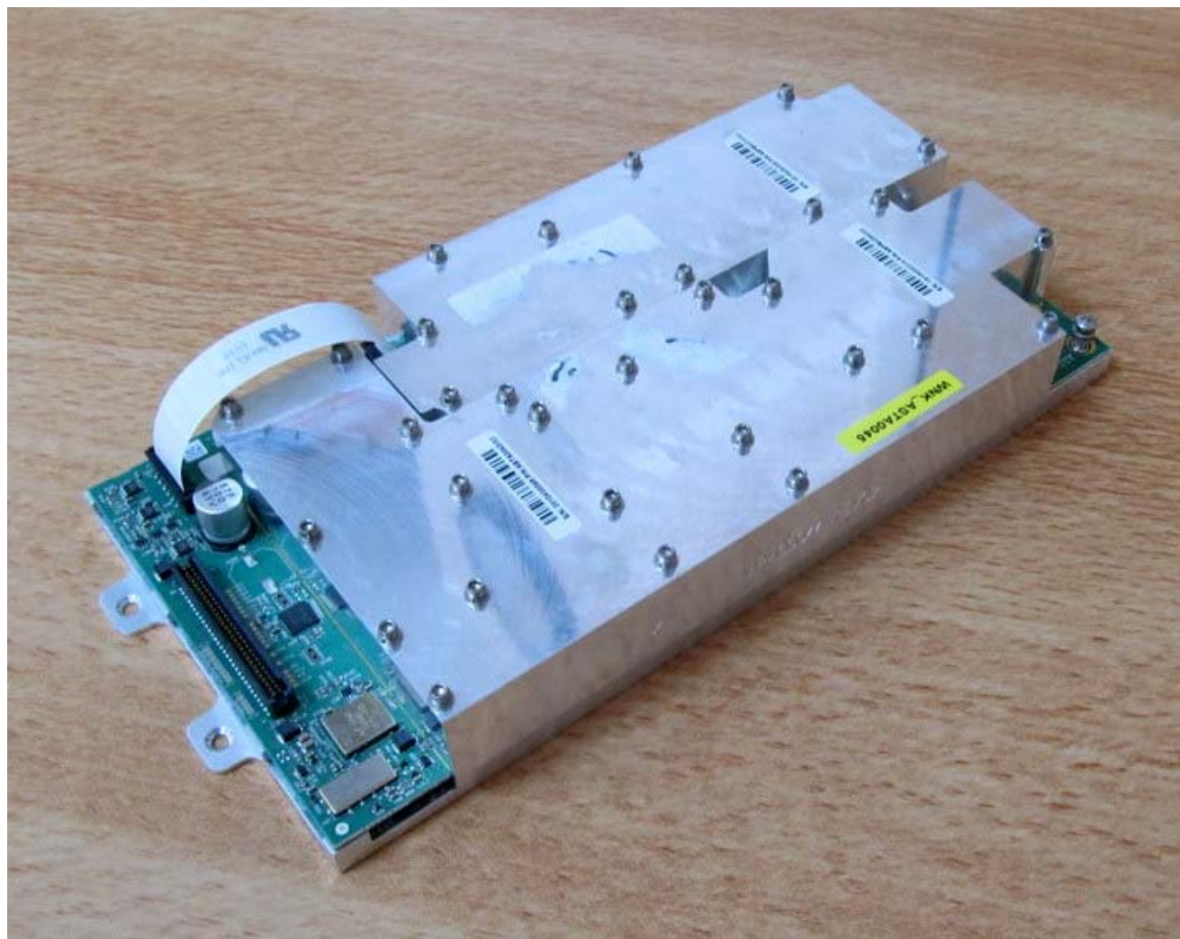
Photograph No.11 RF Board – With cover
