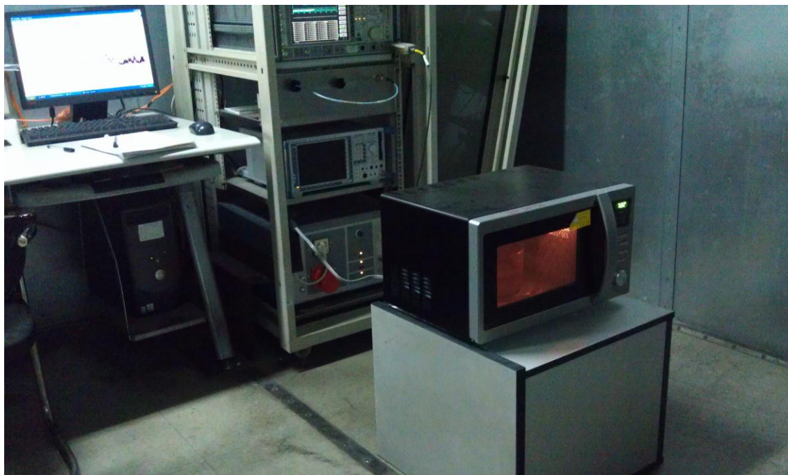
Conducted Emission Test Set-up
