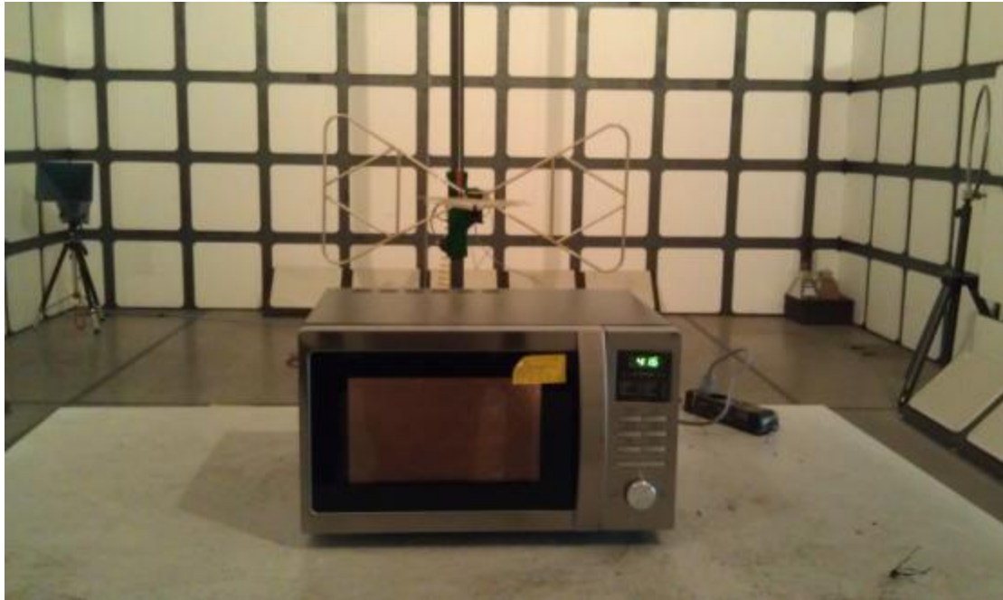
Radiated Emission Test Set-up (30 -1,000MHz)
