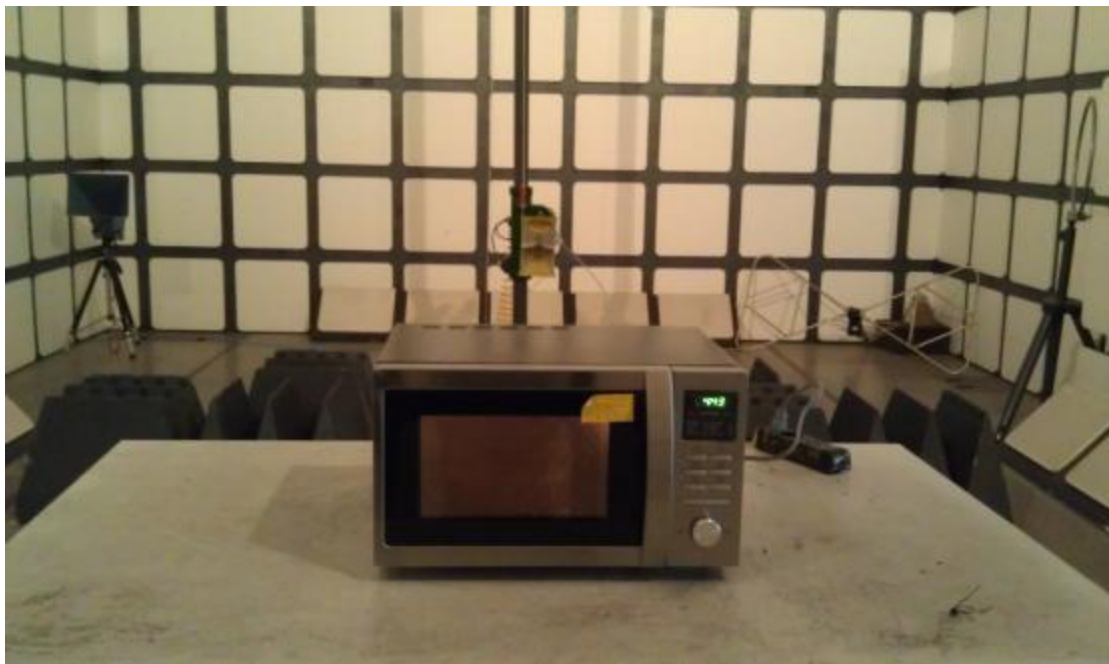
Radiated Emission Test Set-up (1-25GHz)
