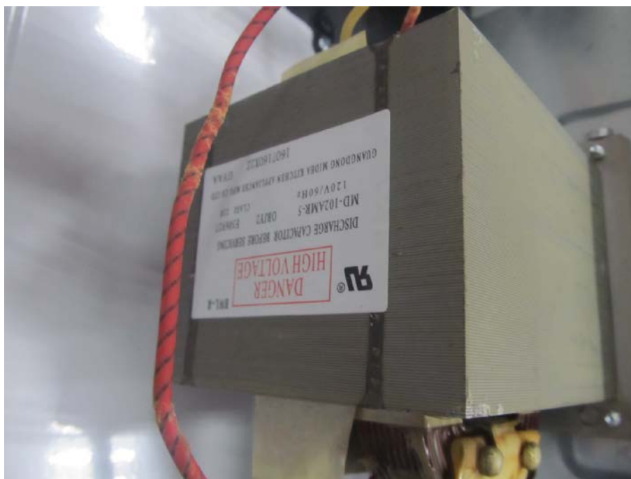
High-voltage Transformer view
