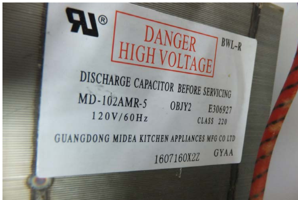
High-voltage Transformer view
