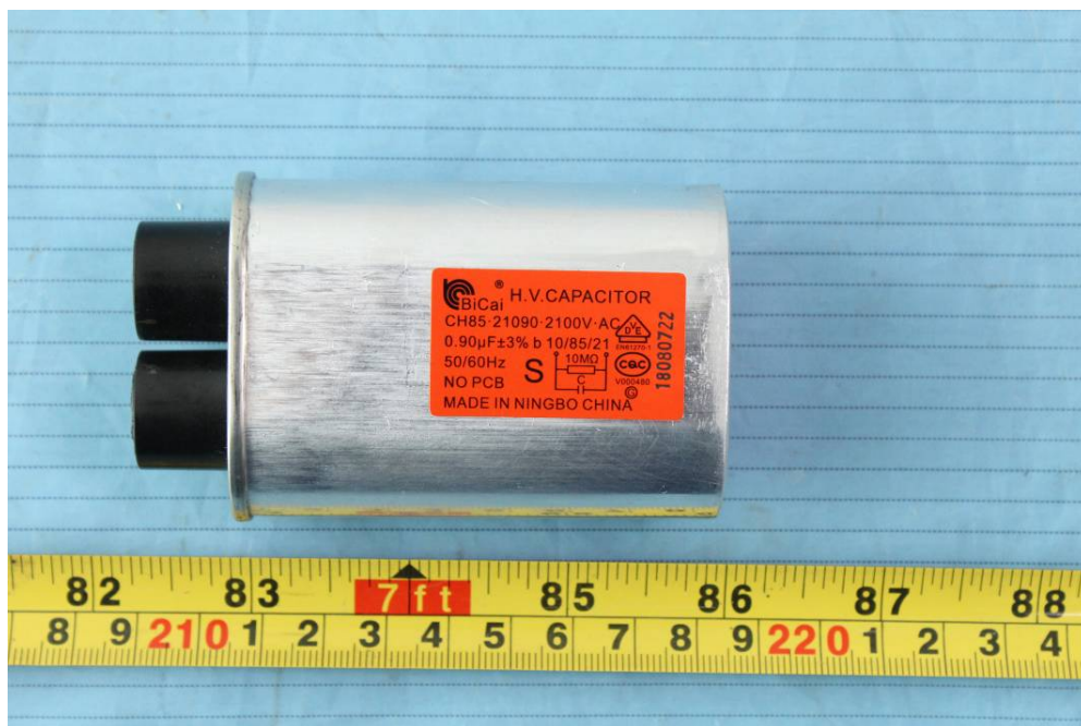
EUT –High Voltage Capacitor View
