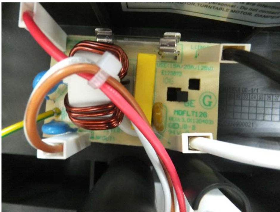
Power Filter Board Top View
