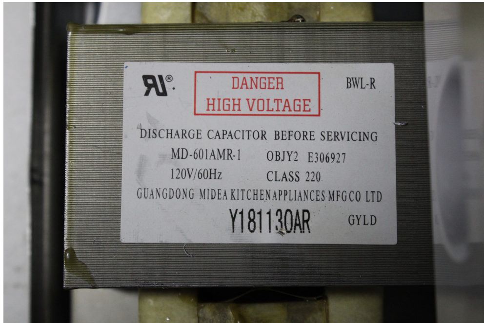
EUT – Transformer View
