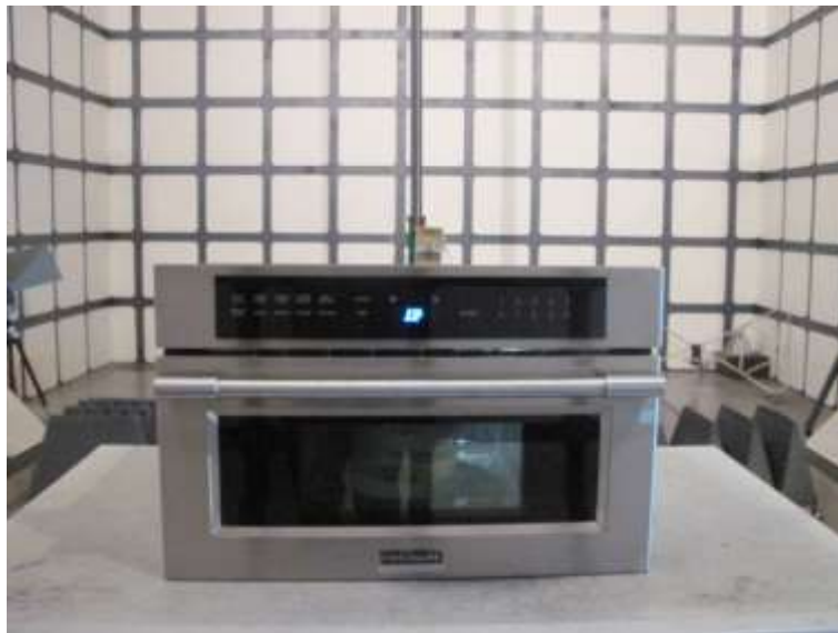
Radiated Emission Test Set-up (1-25GHz):
