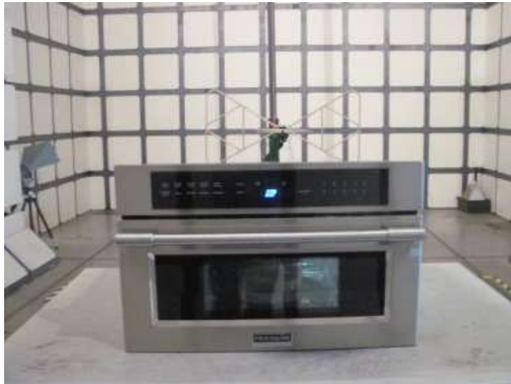
Radiated Emission Test Set-up (30-1000MHz):
