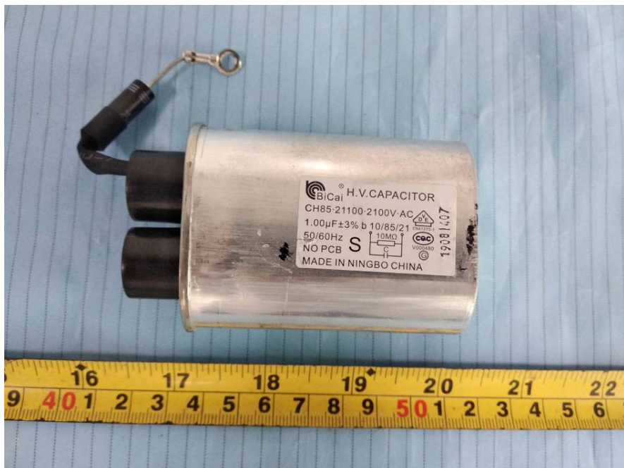
EUT – H.V. Capacitor Top View
