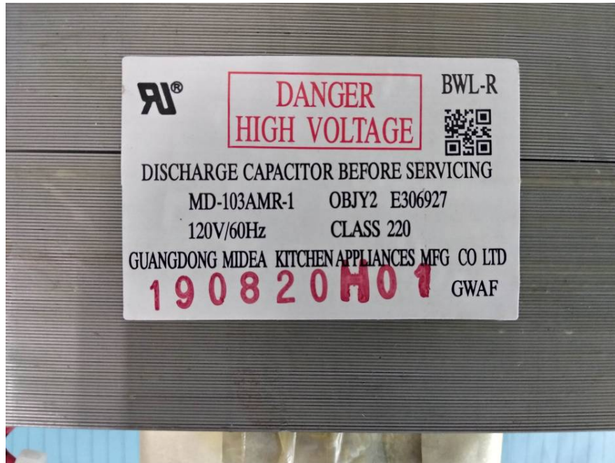
EUT – Transformer Label View
