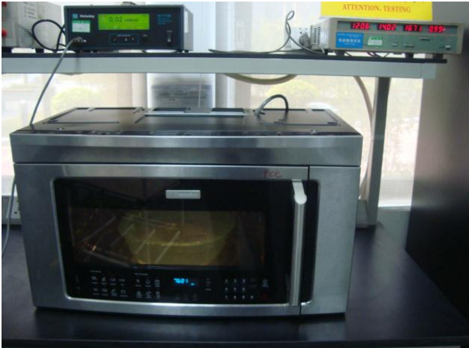
Radiation Hazard Test Set-up
