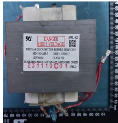
Original high-voltage transformer
