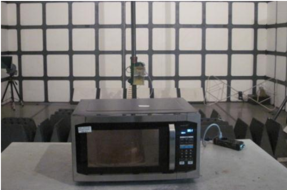
Operating Frequency Test Set-up
