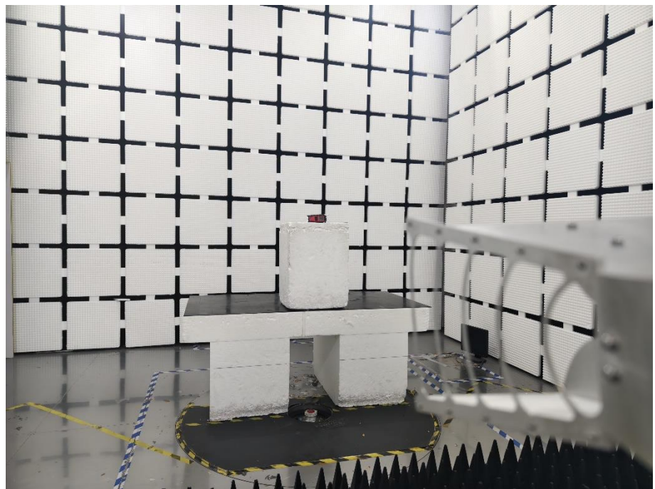
Radiation Emission Test Setup (1GHz to 18GHz)
