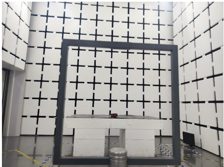
Radiation Emission Test Setup (Below 30MHz)
