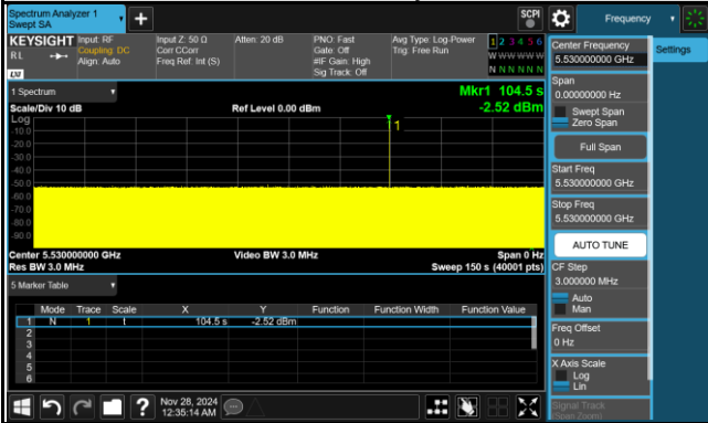
Radar Burst at the End of the Channel Availability Check Time
