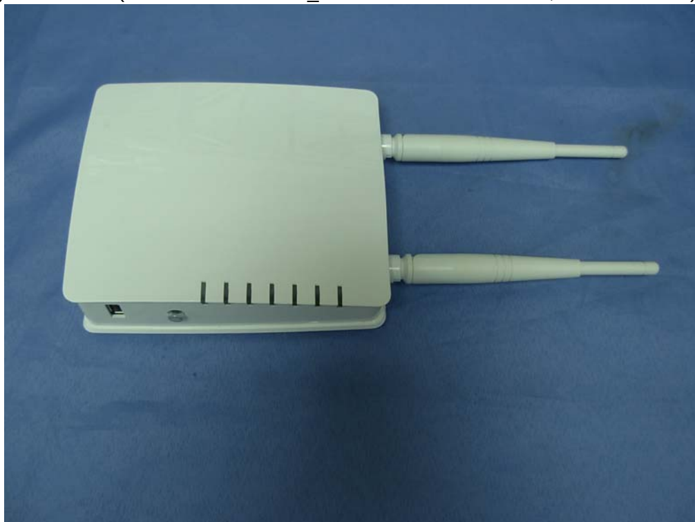
(16) EUT Photo (Antenna: Walsin / PI_RFDPA131307NNAB301 , EUT: FLY-215 )
