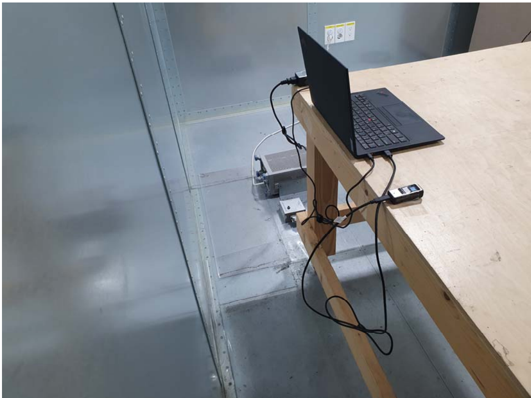
AC power line conducted emission
