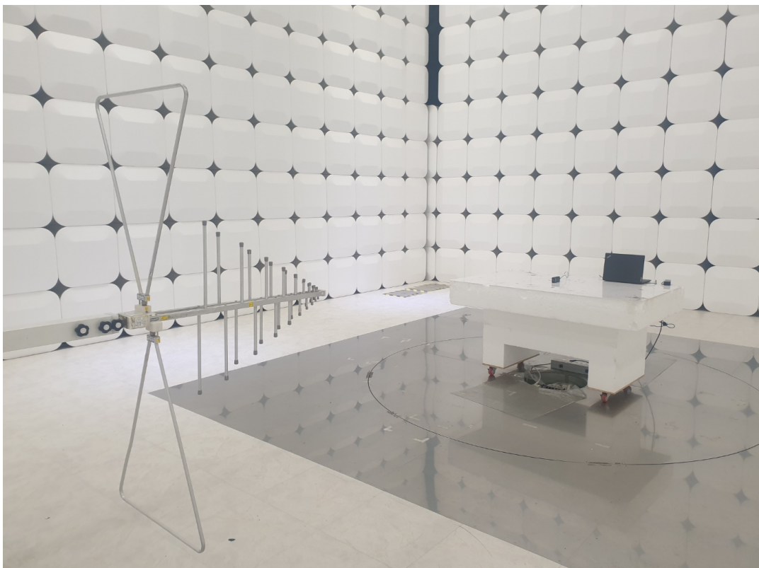
Radiated emission test (30 MHz to 1 GHz)
