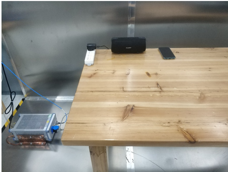
Photograph 3: Set-up for Conducted Emission on AC Mains
