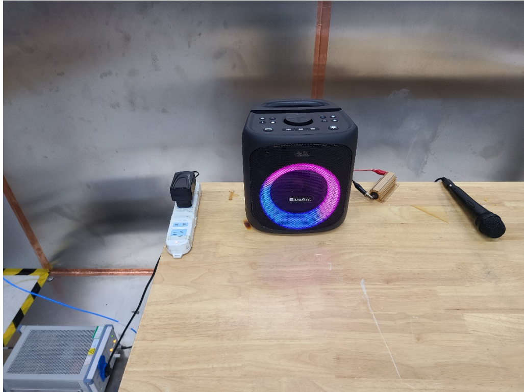
Photograph 3: Set-up for Conducted Emission on AC Mains
