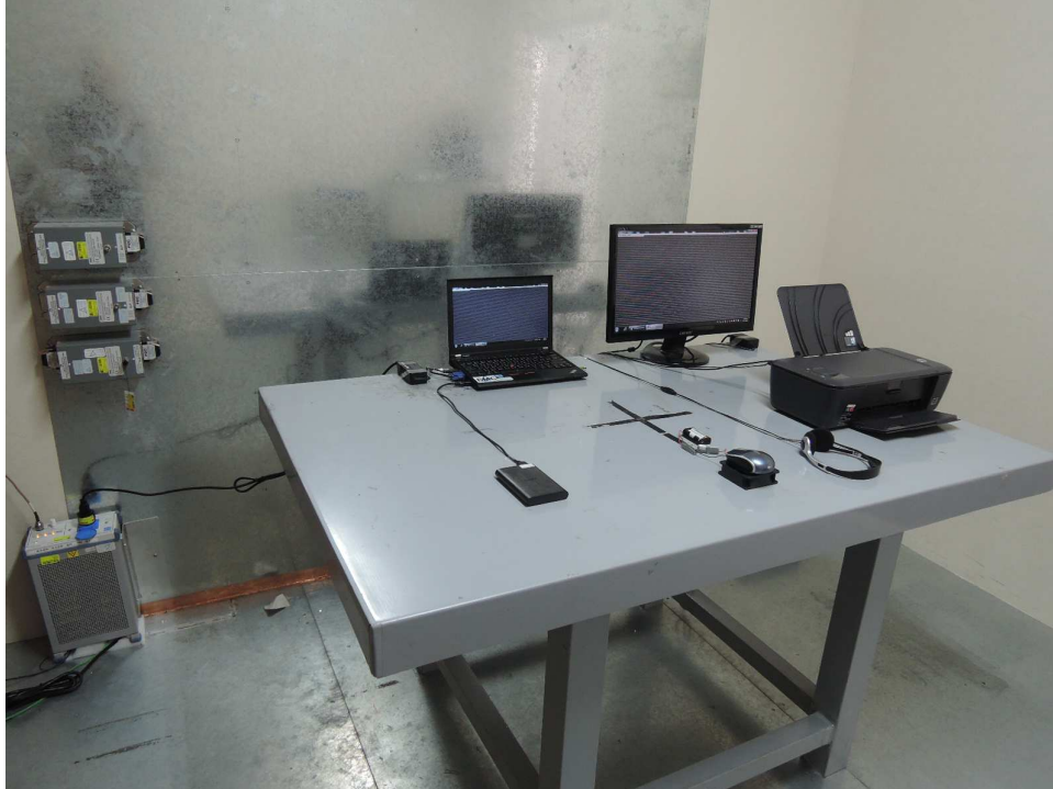
Photograph 6: Set-up for for Mains Conducted testing Front
