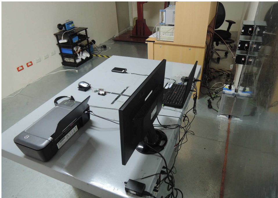
Photograph 5: Set-up for for Mains Conducted testing Back
