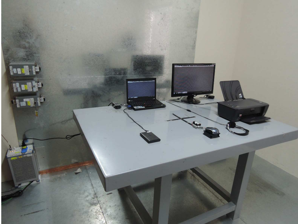
Photograph 6: Set-up for for Mains Conducted testing Front
