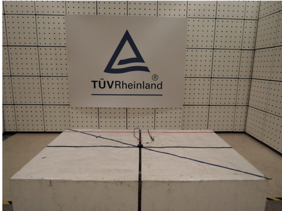
Photograph 1: Set-up for Spurious Emissions (Front View)
