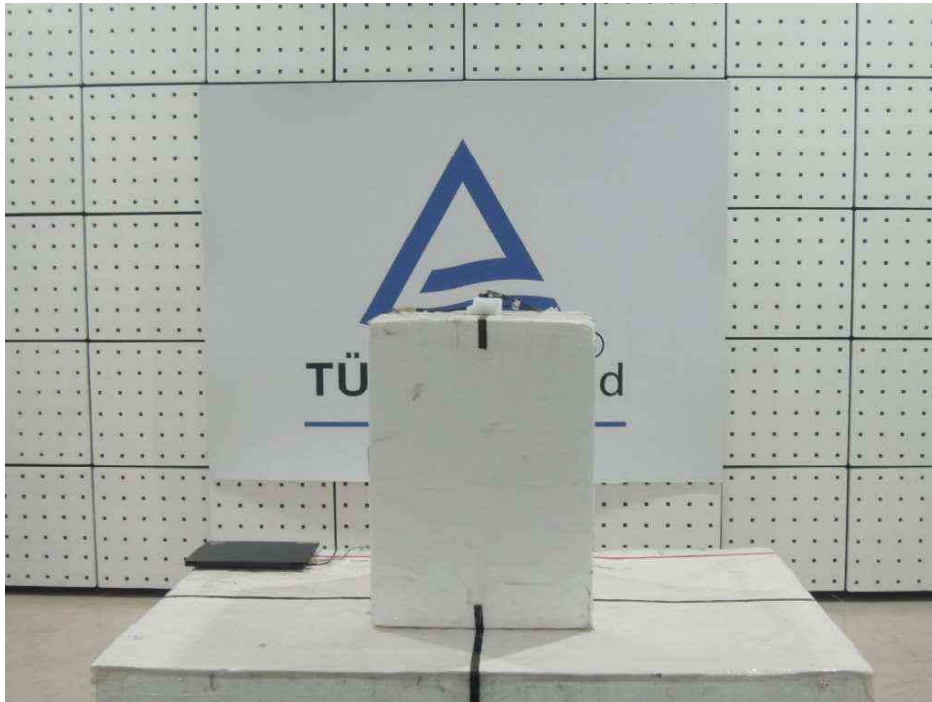
Photograph 9: Set-up for Spurious Emissions (Back View 1) – Right Ear
