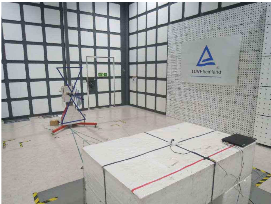
Photograph 9: Set-up for Spurious Emissions (Back View 1) – Right Ear
