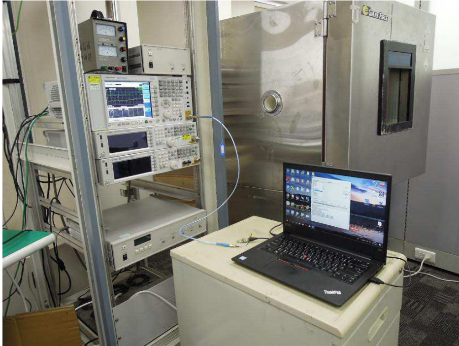
Photograph 13: Set-up for Conducted testing
