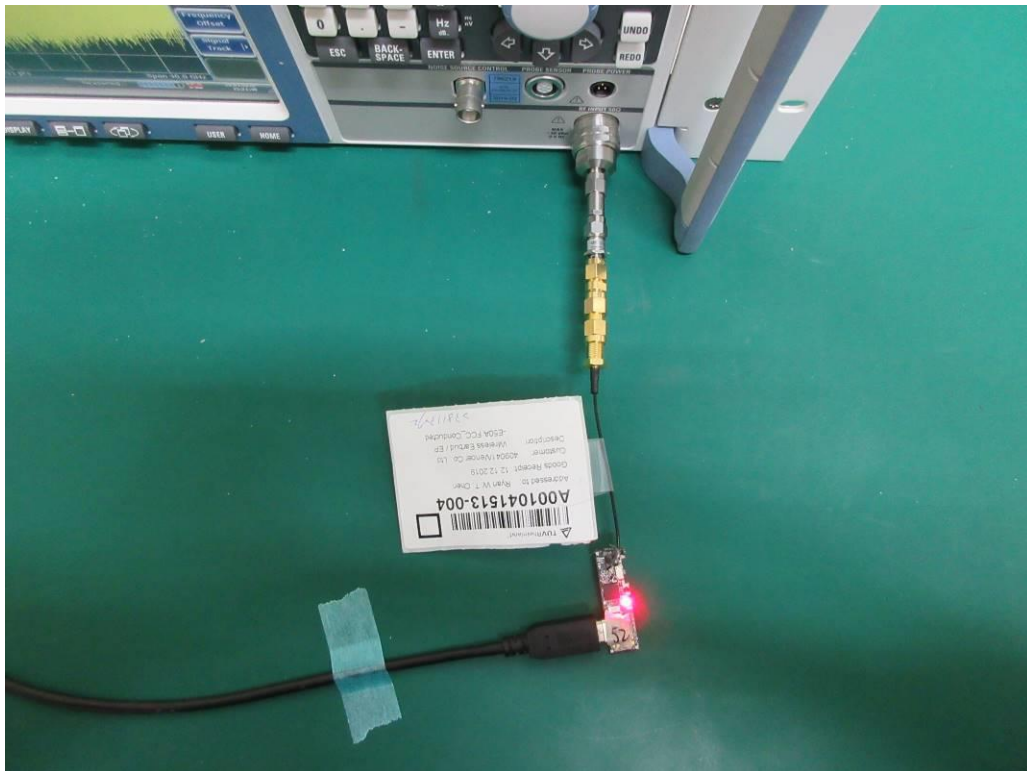
Photograph 7: Set-up for Conducted testing (View 1)
