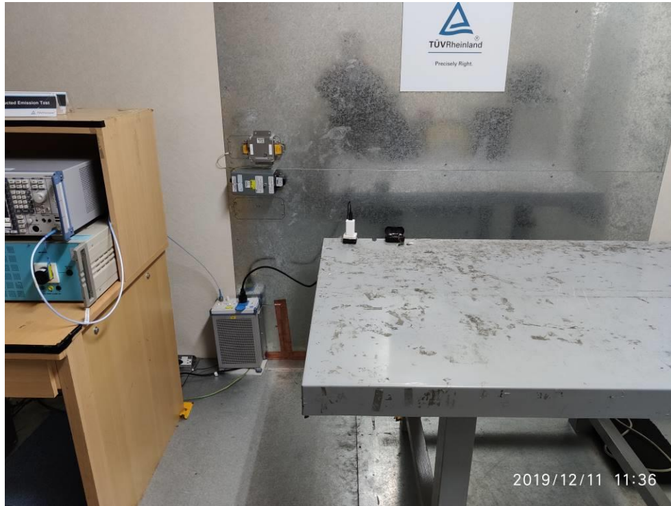
Photograph 9: Set-up for AC Mains (Front View)
