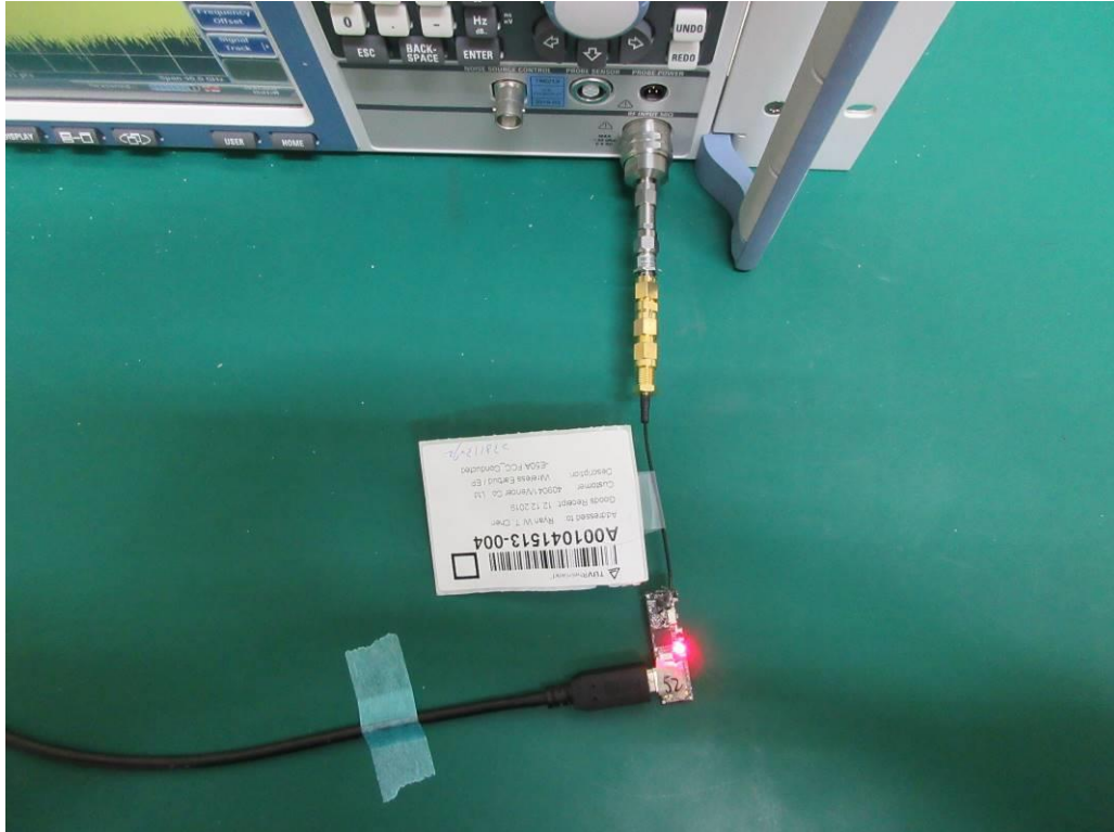
Photograph 7: Set-up for Conducted testing (View 1)
