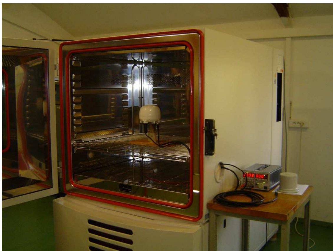
Position of the equipment in the climatic chamber
