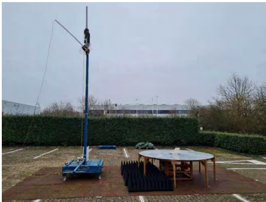
Antenna Characteristics – Configuration 2 Dipole
