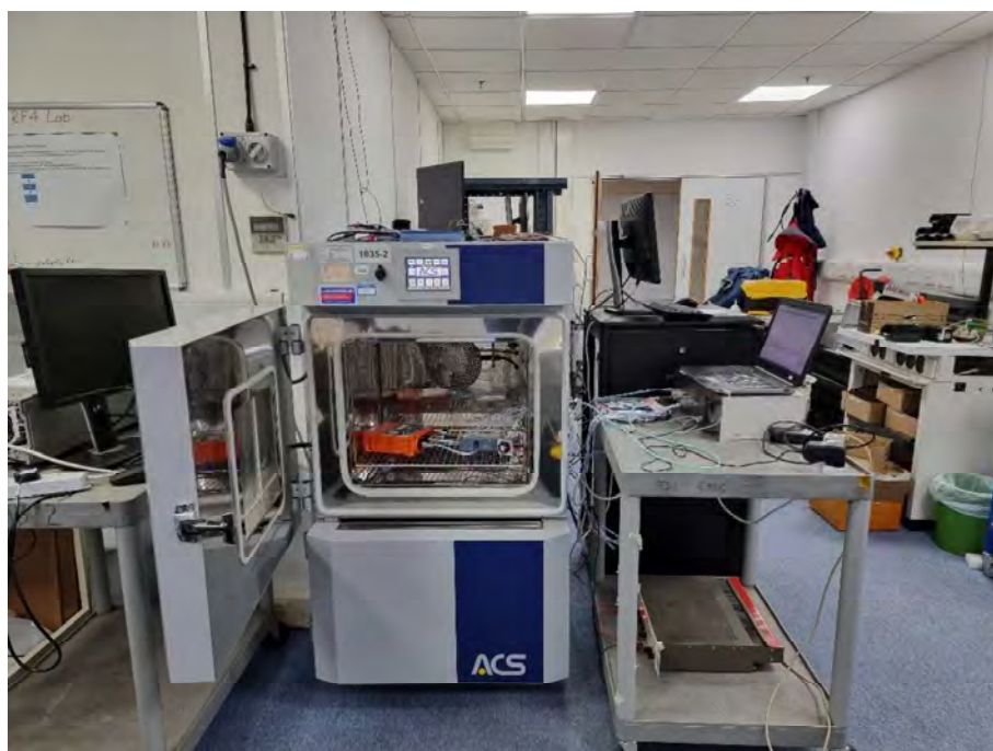
Test Configuration for Conducted RF Tests (EUT, RCP and Buzzer placed in Climatic Chamber for temperature tests)
