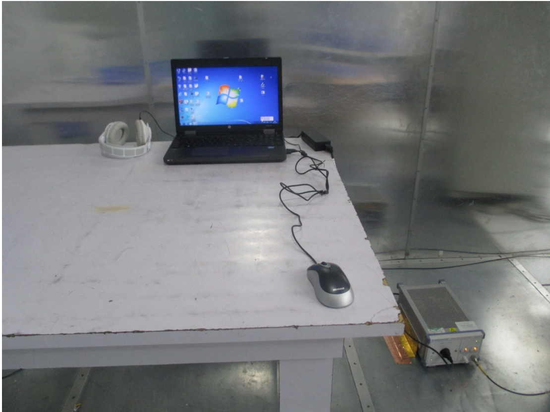
Conducted Emission Test setup photos
