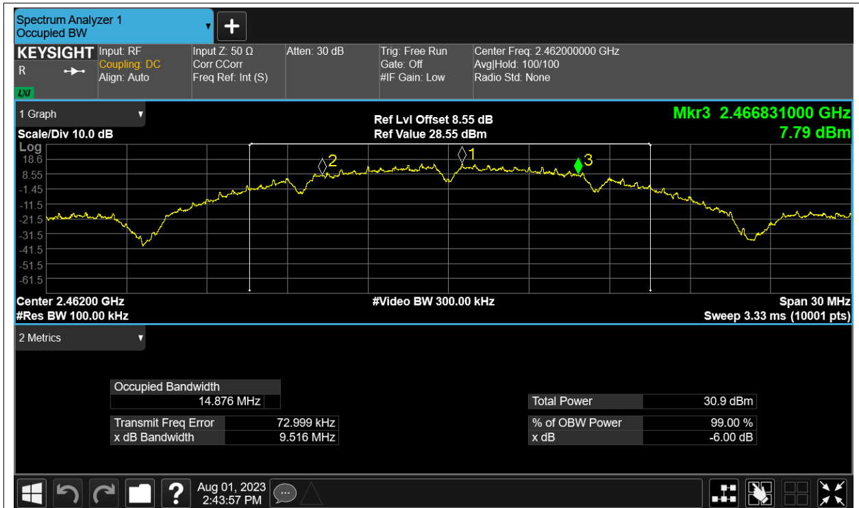
-6dB Bandwidth NVNT b 2412MHz Ant2
