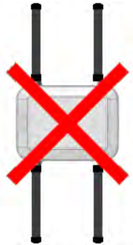
Figure: Incorrect Antenna Placement
