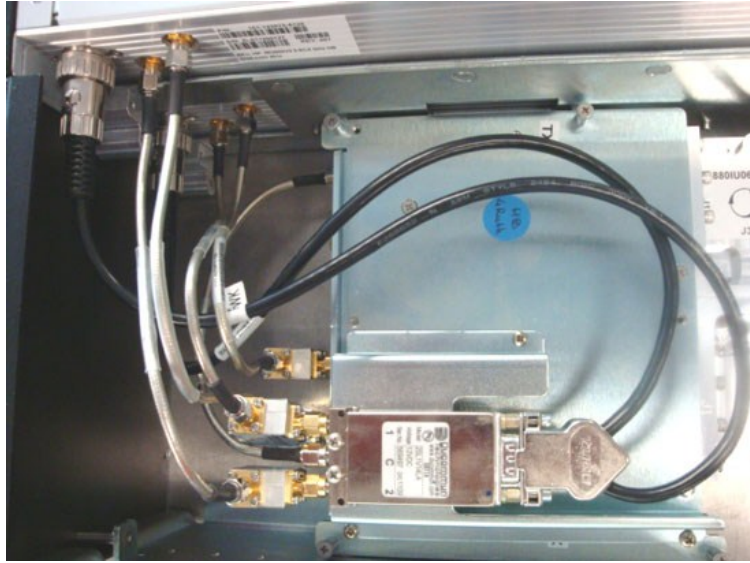
Figure 2-5. IRU 600v3 Tx Switch and RFUv3 Connections
