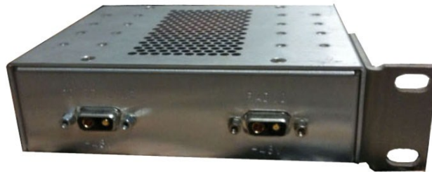
Figure 3-4. Power Line Filter with Bracket
