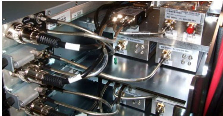
Figure 2-5. IRU 600v3 Tx Switch and RFUv3 Connections
