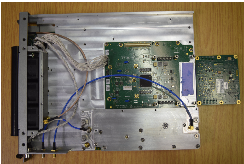
Photo 4, IRU 600v4 RFU DC power board removed:
