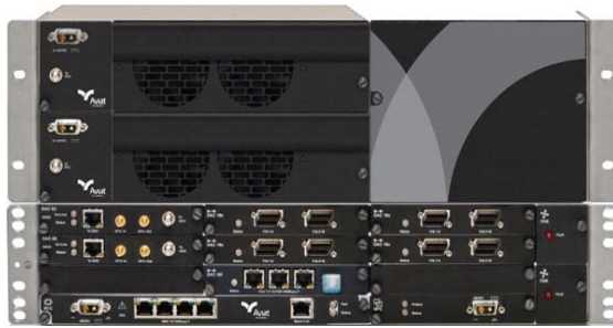
Figure 1. INUe with High-Power 3RU IRU 600
