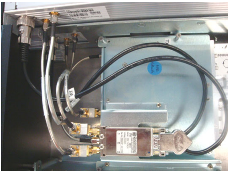
Figure 38. IRU 600v2 Tx Switch and RFUv2 Connections
