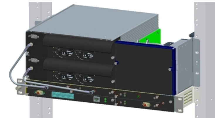
Figure 38. IRU 600v2 Tx Switch and RFUv2 Connections
