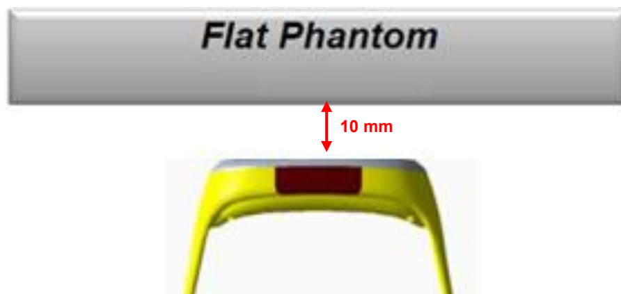
Fig-4.2 Illustration for Face Exposure Setup
